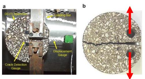
Direct Compact Tension (DCT) (ASTM D 7313)
